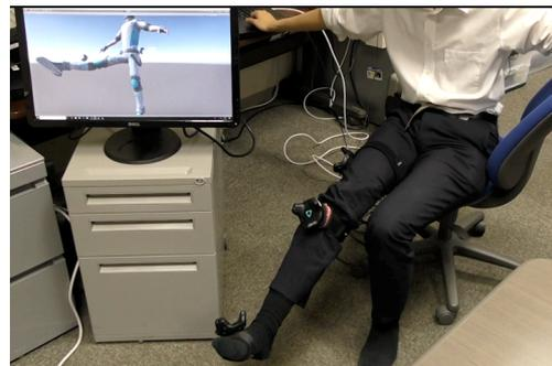
Fig. 2. An occupational therapy system using myoelectric sensor
