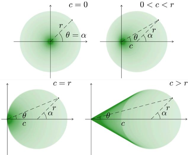
Fig. 3. The relationship between the amplitude ( $r$ ) and the parameter ( $c$ ) that warps the phase ( $\alpha$ ) into the angle ( $\theta$ ) [3].
