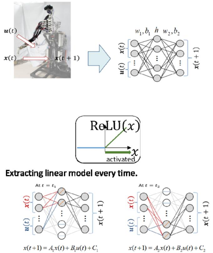
Fig. 2. A neural network for learning the forward dynamics of the muscular-skeletal humanoid upper-body. It has a restricted linear unit (ReLU) as activation function of the middle layers. The ReLU enable to pick the activated unit at the time, and derive linear state equation.
