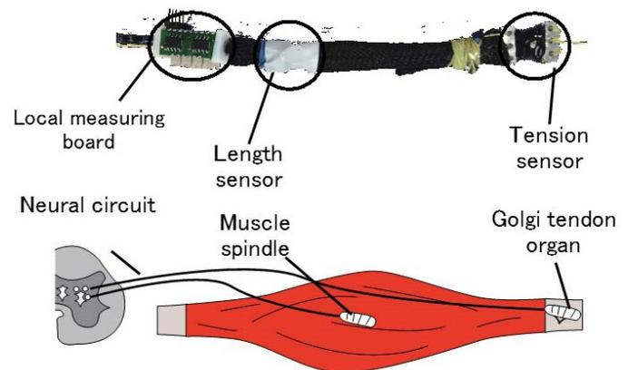
Fig. 1 Proprioceptive sensor board for pneumatic artificial muscles.
