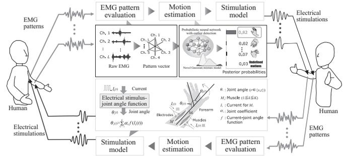
Fig. 1. Concept of the proposed EMG-based human-human interface using FES
