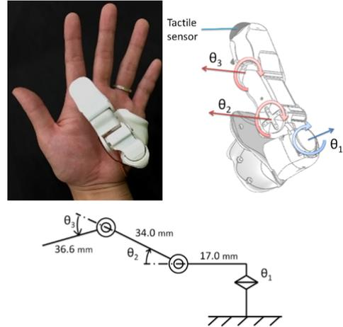
Fig. 1. Extra Robotic Thumb
