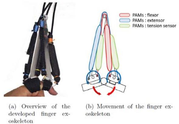
Fig. 3 Master-slave finger exoskeleton driven by pneumatic artificial muscles
