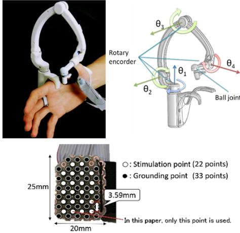
Fig. 2. Manipulation interface for robotic thumb
