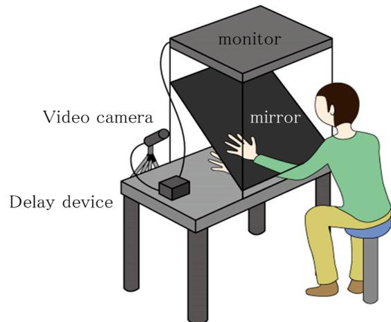
Fig. 1 Visual feedback delay system
